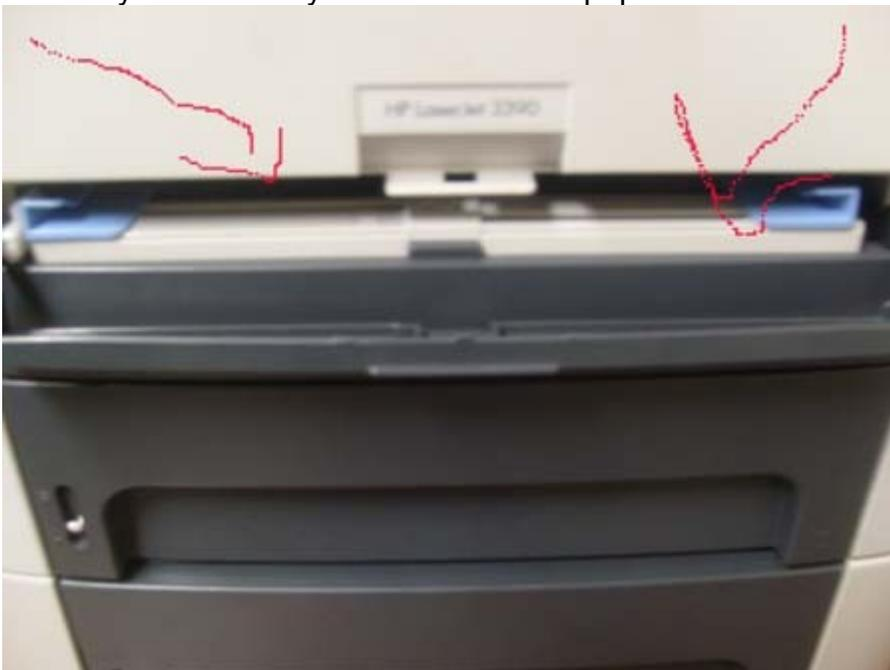
To use that tray you slide a piece of paper straight between the blue guides. Stop when you hear a sound from the printer and feel the machine grab the page. Paper will not go in
