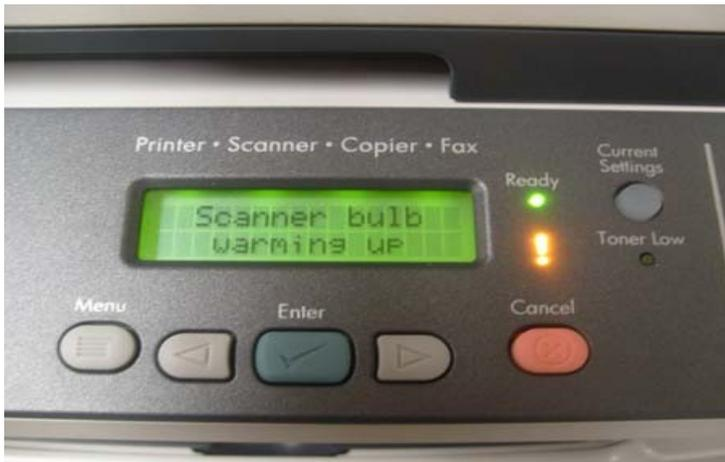
Error messages may be displayed on the screen. (Paper jam, for instance.) There are also indicator lights. If the orange exclamation point is lit and blinking it means there is a problem such as the printer being out of paper. Always check for paper before you try to print.
